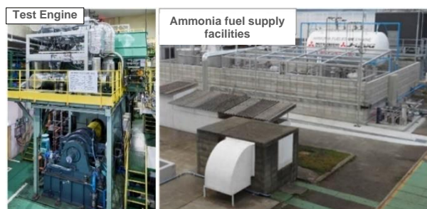
Figure 5. Ammonia-fueled test engine, Ammonia fuel supply facilities
