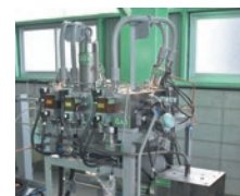
Hydrogen injection unit
