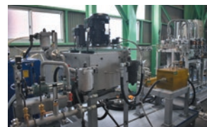
Hydrogen injection test bench
